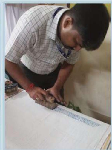
Block printing on cotton fabric
