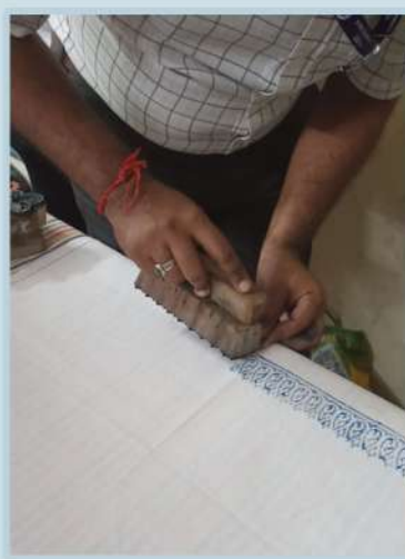
Block printing on cotton fabric
